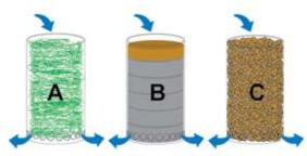
Filtration methods: A fine nylon filter floss for use with a liquid lanthanum preparation; B the suggested filter pads with lanthanum coating on the fibers (see text), followed by fine filter pads; C the suggested granulate with lanthanum coating (for example lanthanum carbonate, see text).
