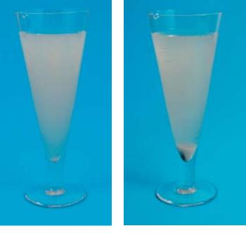
The filtrate was rinsed out of the floss into a glass – within a few minutes a significant layer of sediment had accumulated at the bottom.
