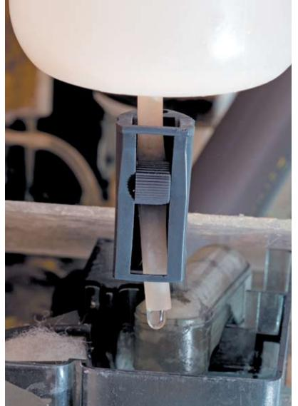
**Experimental addition** of diluted lanthanum chloride solution to an external filter filled with filter floss, feeding into a chamber of a filter tank containing a protein skimmer; within seconds of the beginning of the addition of lanthanum the skimmer overflowed. The drip rate was regulated using a dosing clamp, such as is used for medical infusion, on the feeder tube.
