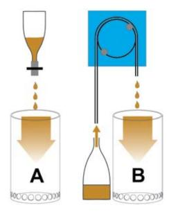
The addition of lanthanum to the proposed lanthanum filter: A dropper bottle with airline tubing and clamp; B dosing pump with clamped tube.
