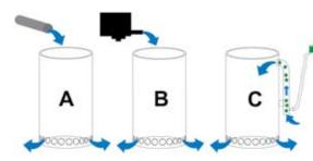
Feeding water to the suggested lanthanum filter: A via an existing supply pipe (eg branch from an outflow pipe, branch from return pipe, inter alia); B via a very low-turnover powerhead; C via an airlift.
